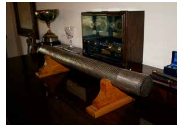
First piece of locked coil winding rope hand made by Telford Clarence Batchelor and Henry Herbert Horsfall, 1885
